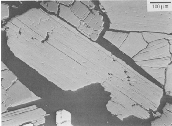
Figure 3. Secondary electron image of oxidized biotite in thin section from the interior of a subsurface boulder.
