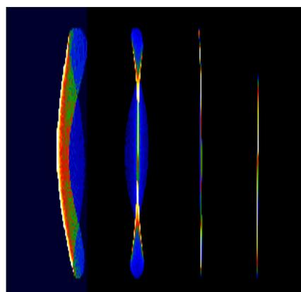
FIG. 2. Calculated spectral aberration figures from an isochromatic figure. The figures from left to right correspond to increasing orders of aberration correction from partial 2<sup>nd</sup> order up to 4<sup>th</sup> order.
