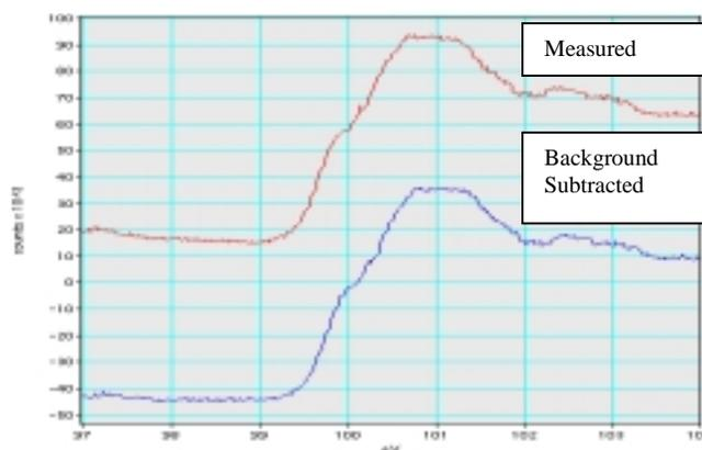
FIG. 3 Si spectrum collected with a 2 mm aperture at 200 kV on a monochromated TF20.
