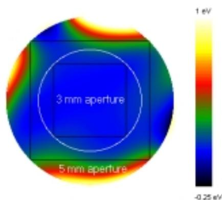
FIG. 1. Isochromatic surface of the 4<sup>th</sup> order corrected aberrations with the new spectrometer. The square inside the circle represents the image captured on the square CCD detector. All data outside of the outer square has been extrapolated.
