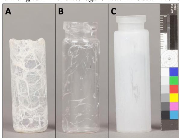
Figure 1. The three vials chosen for cross-sectioning and analysis. These vials represent a range of alteration responses from extensive cracking and vial failure (A) to larger scale cracking of otherwise clear glass (B), to increased opacity with no obvious fracturing (C). Image credit: Keats Webb, MCI.
