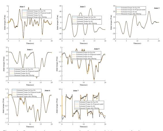
Figure 4. Comparison between the measured and estimated joint torques for the parameter identification.
