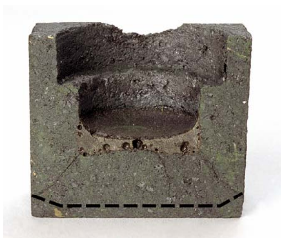
FIG. 1: Fired cup test with slag penetration.
