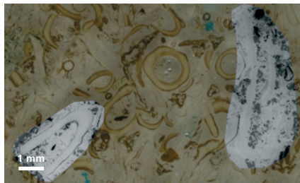
Using ZEISS Atlas 5 software, a light microscope overview image (brown) is correlated with high resolution SEM images (gray) for a fossiliferous carbonate sandstone sample. Sample courtesy of D. Schumann, Fibics Incorporated, Ottawa, Canada.
