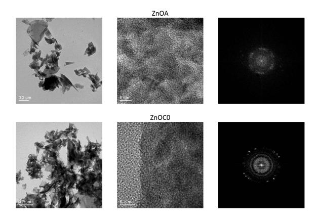
**Figure 1.** Identification of the morphology obtained in the three different routes of synthesis with NaOH precipitant ZnOA0 and KOH for ZnOC0.
