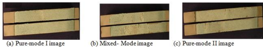
Figure 1. Failure surfaces observed visually under different mode conditions
