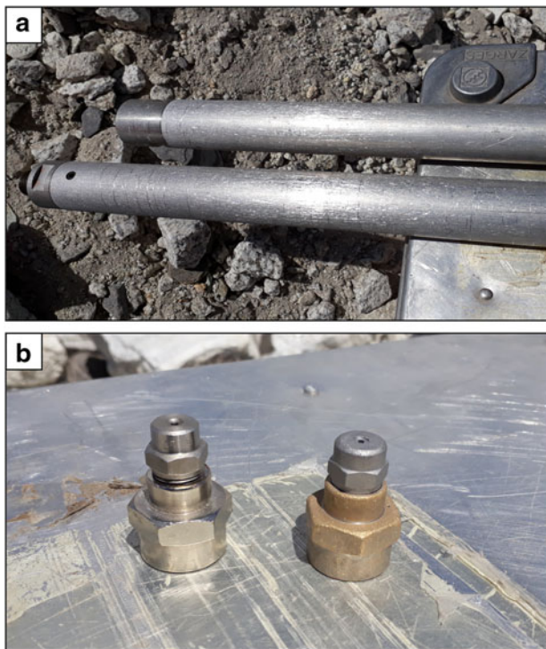
Fig. 4. Images of drill equipment wear from contact with englacial debris. (a) Drill stems showing abrasion; (b) drill nozzles (unused on the left and used on the right). Note the chrome plating has worn completely from the used reducing bush on the right.
