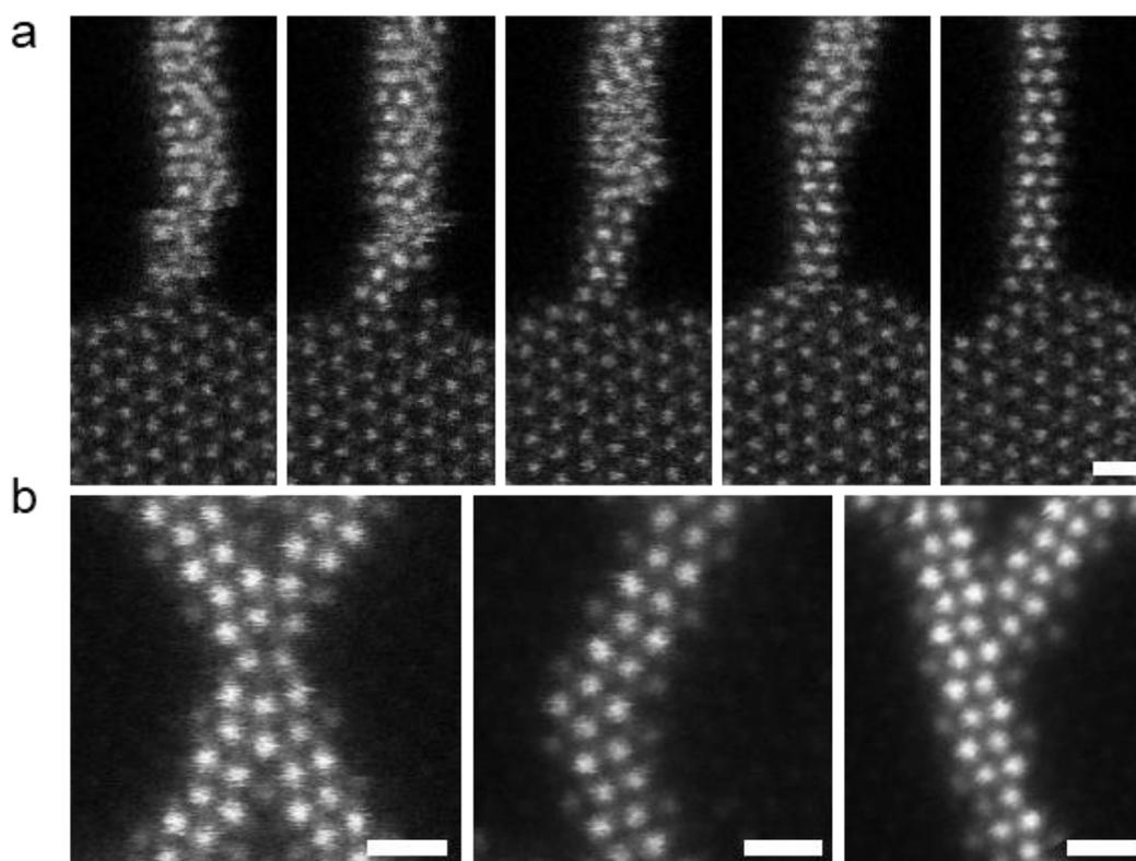
**Figure 1:** *In-situ* fabrication of nanowires from a TMDC monolayer and different types of junctions. (a) Sequential ADF images showing the fabrication process of an individual MoS nanowire entirely within a semiconducting MoS<sub>2</sub> monolayer. (b) ADF images of different types of nanowires and ramified junctions created by advanced control of the electron irradiation inside the STEM, demonstrating the diversity of building blocks made from these nanowires. Scale bars: 0.5 nm.
