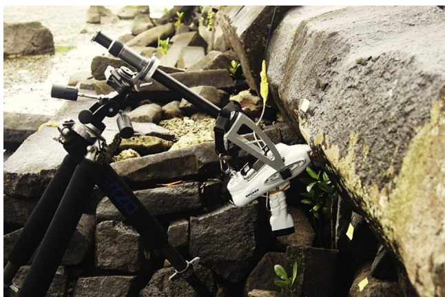
Fig. 6. Portable XRF assaying columnar basalt in the field. The pXRF was used on islets across the site of Nan Madol and intensively on the islet of Nandauwas. Photo credit: Mark McCoy.
