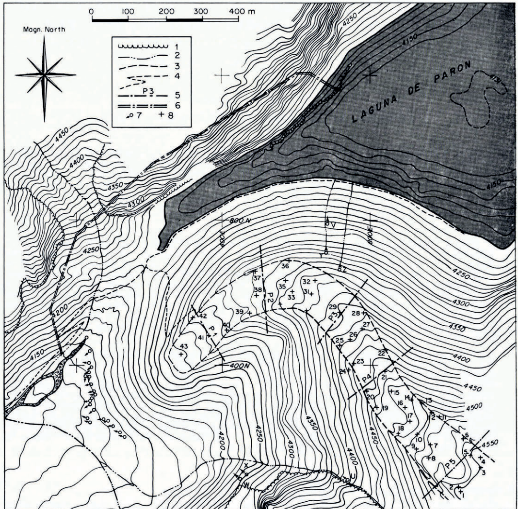
Fig. 1. Map of the area, as surveyed by CPS. 1 = limit between bare rock and scree; 2 = streams; 3 = limit of debris-covered glacier; 4 = mule tracks (there is an earth road to the tip of the lake by now); 5 = conductivity profiles; 6 = tunnel under construction; 7 = springs; 8 = marks on big boulders which were surveyed.
