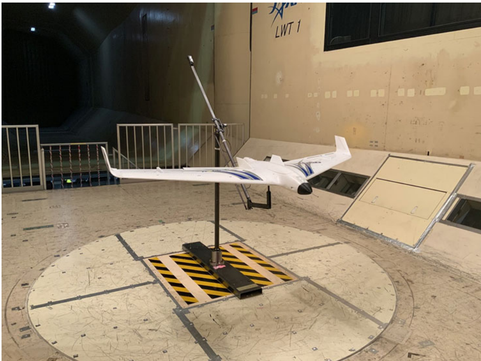
Figure 6. The picture of dynamic wind tunnel testing model. The safety fences are temporary installations set up in preparation, so they are removed during actual airflow testing.
