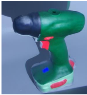
b) Spatial Augmented Reality Prototype using SPARK. Colour is projected onto a blank 3D version of the product.
