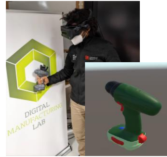
c) Prototype using a virtual reality overlay on top of a blank 3D version of the product.
