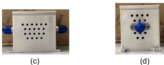
Figure 6. Sensors with the adjustable cavity. (a) Straight sensor with adjustable cavity but without shielding cover. (b) Meander sensor with adjustable cavity but without shielding cover. (c) Front view of the meander sensor with shield cover. (d) Side view of a meander sensor with shield cover.
