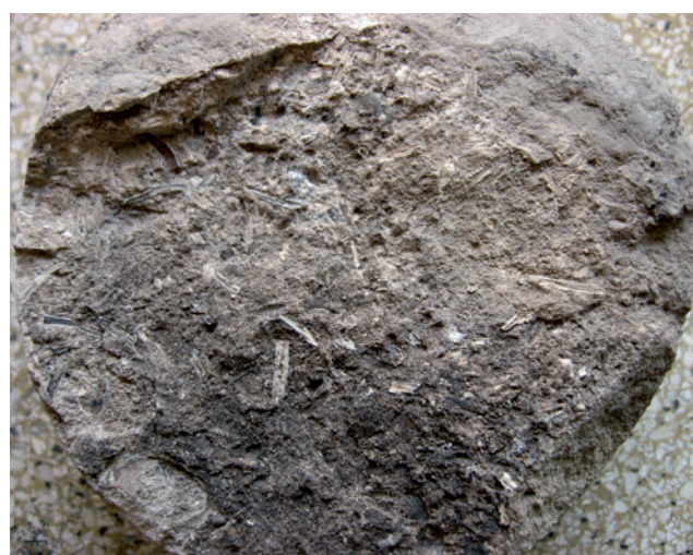
Fig. 11. Serpulid bed, stained by lignite that migrated downwards from overlying Cenozoic Opglabbeek Formation (not preserved in situ as stratiform unit) through porous fine-grained calcarenite at a depth of 708.13 m (top Chalk Group at 703 m) in the Turnhout borehole (core diameter 8 cm).
