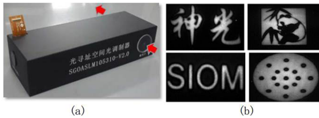
Figure 17. (a) Physical photograph of the optically addressed liquid crystal spatial light modulator and (b) demonstration of near-field spatial intensity control.
