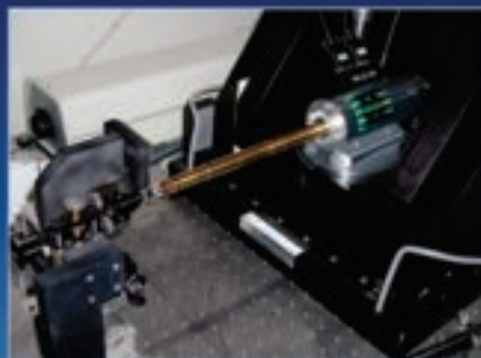
Capacitive transducer within TEM holder undergoing interferometric calibration
