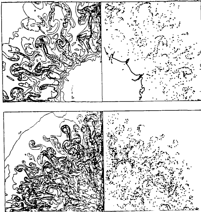
FIGURE 1. Density contour (left) and positions of marker particles (right) on 1025 \times 1025 grids for type II-P supernova explosions. (a) IIP20 (upper): Time after the explosion is 8 \times 10^5 s. The size of the computational box is 1.65 \times 10^{14} cm ( 2400 R_{\odot} ). (b) IIP13 (lower): Time after the explosion is 3 \times 10^5 s. The size is 6.8 \times 10^{13} cm ( 980 R_{\odot} ).
